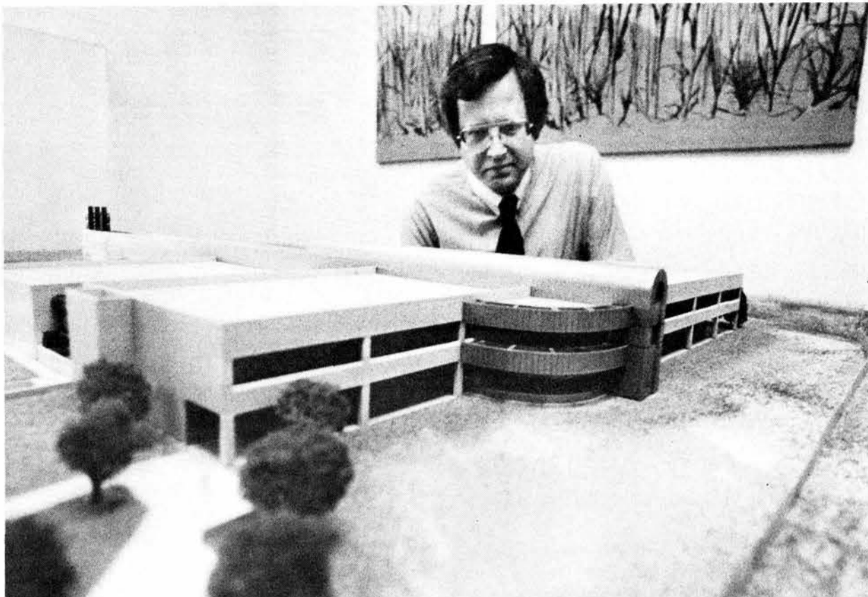
ENGINEERING MODEL of Sandia's new RHIC laboratory is examined by Doug Weaver (2102), RHIC technical manager. The model gives an idea of the way the two-story, multi-sectioned building will appear when construction is complete in 1987. The 320-foot-wide front section is an office/light laboratory area; the back section is divided into a fabrication clean room, support area, and an ultra-clean, state-of-the-art 12,000-square-foot clean room for wafer fabrication. A utility spine connects the two sections with a skylight area over the front. Architect firm for the $40.5 million project is Anderson, DeBartolo, Pan, Inc. of Tucson.
